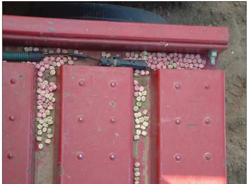
Picture above shows: A closer look at the catwalk of the seeder reveals that treated seeds were left on the machine. The equipment was not cleaned prior to entering the organic field.
